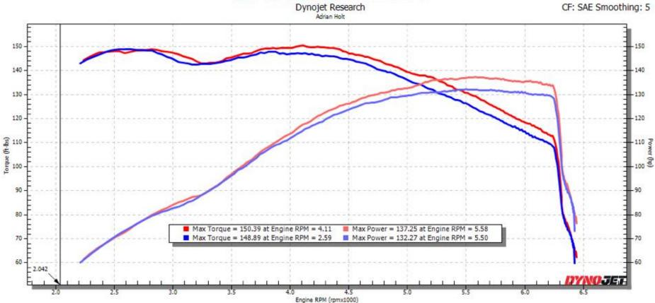
128 Stump Puller, Stock Heads, CR480, SE 55mm intake, 6.2gps inj, Freedom 2-2
